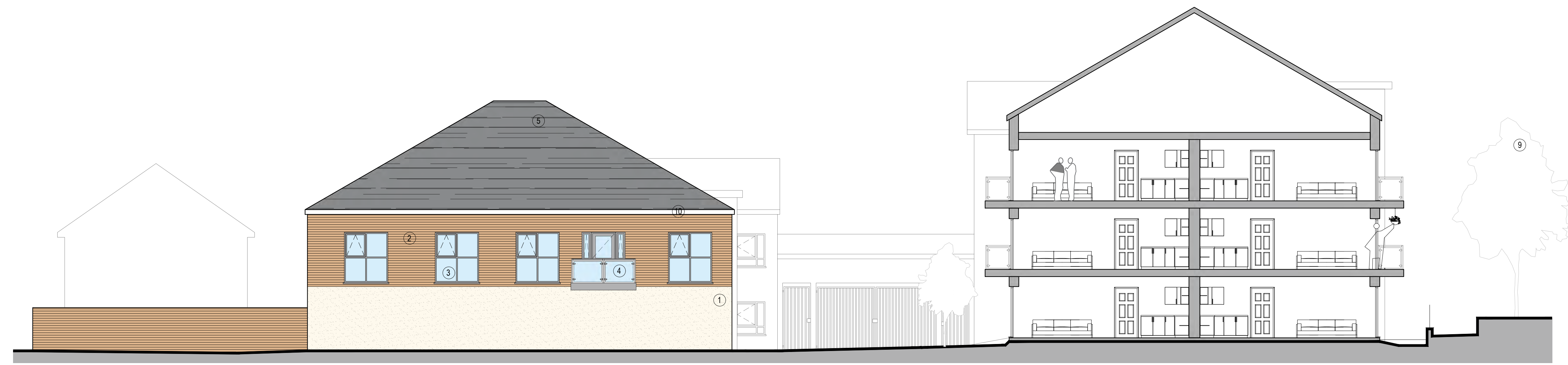
03 Proposed Inner Courtyard Elevation
